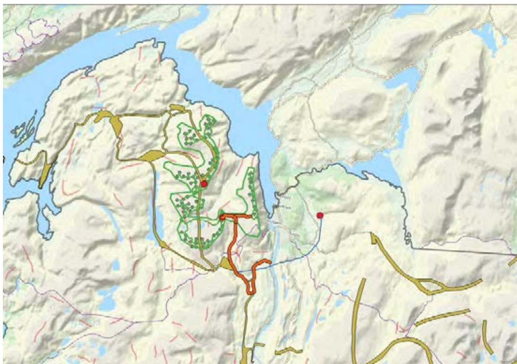
Picture 25 Blue line to the east is a new 132kV power line Middagseidklumpen - Kleivan - Marka. New access road to the wind farm is marked with a red line. Green lines show internal roads and green dots mark wind turbines. Red dots mark transformer stations. A double 132 kV switch field will be installed in the existing Marka transformer station.
